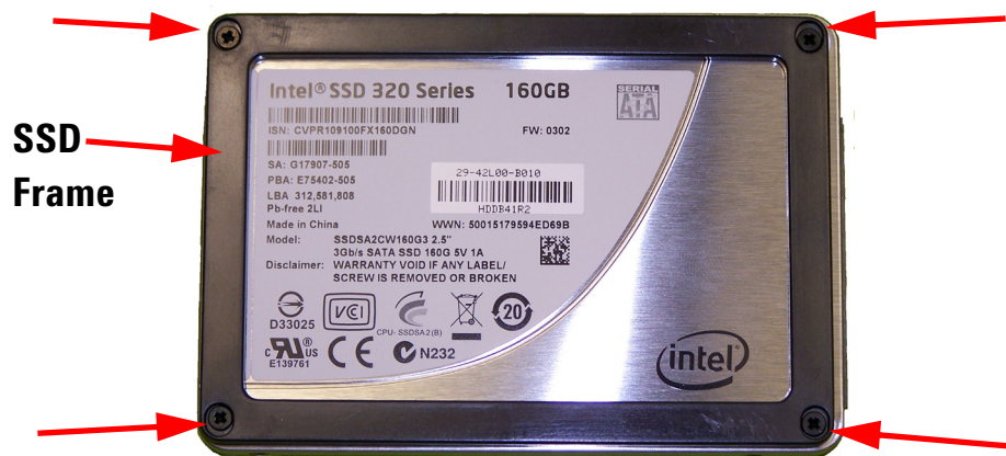
Figure 18 SSD Frame, remove four screws
